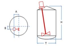
When D/T ratio is too high, you may have impeller very close to vessel wall.
