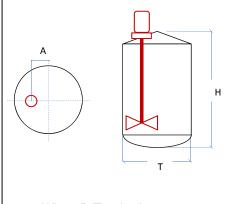
When D/T ratio (between impeller and vessel diameter) is < 0,3, it is possible a vertical off set installation, with  $A=0,16\div0,25\ T$
